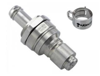
Koolance patented quick disconnect no-spill coupling with automatic shutoff. 6mm (1/4in) ID male panel-mountable hose barb with clamp for 10mm (3/8in) OD. It will only fit a Koolance QD2H female quick disconnect.
