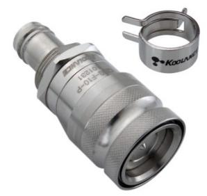
Koolance patented quick disconnect no-spill coupling with automatic shutoff. 10mm (3/8in) ID female panel-mountable barb fitting with spring clamp for 13mm (1/2in) OD. It will only fit a Koolance QD3 male quick disconnect.
