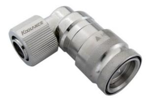
Koolance patented quick disconnect no-spill coupling with automatic shutoff. 10mm (3/8in) ID female swiveling elbow connection with compression fitting. It will only fit a Koolance QD3 male quick disconnect.
