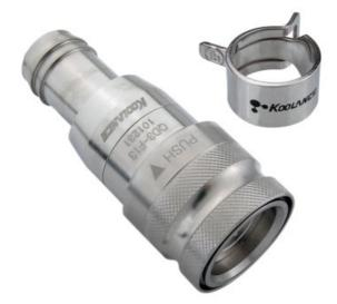
Koolance patented quick disconnect no-spill coupling with automatic shutoff. 13mm (1/2in) ID female barb fitting with spring clamp for 16mm (5/8in) OD. It will only fit a Koolance QD3 male quick disconnect.
