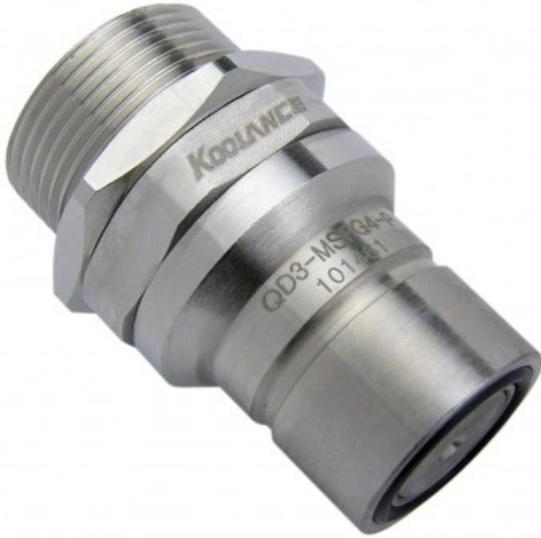
Koolance patented quick disconnect no-spill coupling with automatic shutoff. G 1/4 BSPP (parallel) thread female with panel-mount opposite a male "QD3" quick-disconnect. It will only fit a Koolance QD3 female quick disconnect.
