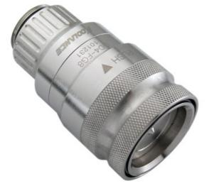
Koolance patented quick disconnect no-spill coupling with automatic shutoff. G 3/8 BSPP (parallel) thread female fitting for screwing directly into a water block or other component of same threading. It will only fit a Koolance QD4 male quick disconnect.
