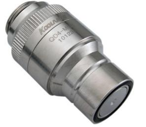
Koolance patented quick disconnect no-spill coupling with automatic shutoff. G 3/8 BSPP (parallel) thread male fitting for screwing directly into a water block or other component of same threading. It will only fit a Koolance QD4 female quick disconnect.
