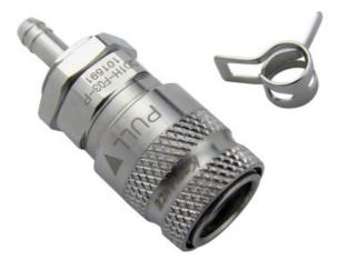
Koolance patented quick disconnect no-spill coupling with automatic shutoff. 3mm (1/8in) ID female panel-mountable hose barb with clamp for 5mm (3/16in) OD. It will only fit a Koolance QD1H male quick disconnect.
