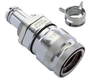
Koolance patented quick disconnect no-spill coupling with automatic shutoff. 13mm (1/2in) ID female panel-mountable barb fitting with spring clamp for 16mm (5/8in) OD. It will only fit a Koolance QDT4 male quick disconnect.
