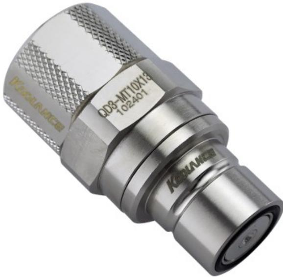
Koolance patented quick disconnect no-spill coupling with automatic shutoff. 10mm (3/8in) ID male straight connection with compression fitting. It will only fit a Koolance QD3 female quick disconnect.
