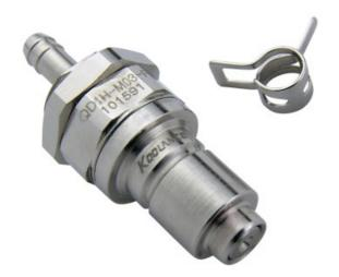
Koolance patented quick disconnect no-spill coupling with automatic shutoff. 3mm (1/8in) ID male panel-mountable hose barb with clamp for 5mm (3/16in) OD. It will only fit a Koolance QD1H female quick disconnect.
