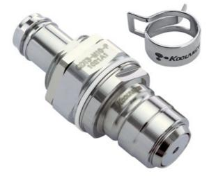
Koolance patented quick disconnect no-spill coupling with automatic shutoff. 10mm (3/8in) ID male panel-mountable hose barb with clamp for 13mm (1/2in) OD. It will only fit a Koolance QDT3 female quick disconnect.
