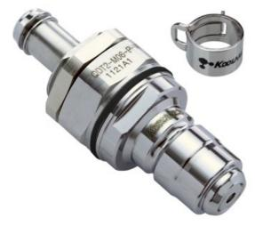
Koolance patented quick disconnect no-spill coupling with automatic shutoff. 6mm (1/4in) ID male panel-mountable hose barb with clamp for 10mm (3/8in) OD. It will only fit a Koolance QDT2 female quick disconnect.
