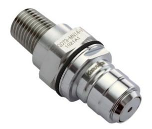
Koolance patented quick disconnect no-spill coupling with automatic shutoff. 1/4 NPT (tapered) threaded male fitting for screwing directly into a component of the same threading. It will only fit a Koolance QDT3 female quick disconnect.
