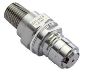
Koolance patented quick disconnect no-spill coupling with automatic shutoff. 1/4 NPT (tapered) threaded male fitting for screwing directly into a component of the same threading. It will only fit a Koolance QDT3 female quick disconnect.
