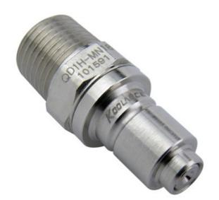
Koolance patented quick disconnect no-spill coupling with automatic shutoff. 1/8 NPT (tapered) male fitting for screwing directly into a component of the same threading. It will only fit a Koolance QD1H female quick disconnect.
