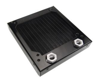
HX-422 is a low profile aluminum radiator designed for one 120mm fan. With a fin density of 18 FPI (fins per inch), it is optimized for quieter air flow ranges. It has a dual pass coolant design, and is G 1/4 BSPP (parallel) thread for hose fittings. 30mm (1.18") long mounting screws are included for 25mm thick fans (see Koolance <u>radiator screw packs</u> for additional options).
