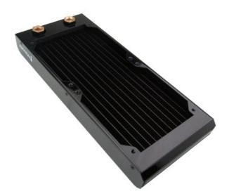
The copper core HX-CU720VS provides an approximate 700W of added heat dissipation when coupled with two 120mm fans. With a fin density of 20 FPI (fins per inch), it is optimized for low to mid-range air flow. Vertical (perpendicular) G 1/4 BSPP (parallel) thread fitting sockets. 30mm (1.18") long mounting screws are included. Dual pass, 15mm (0.59") fan hole spacing.
