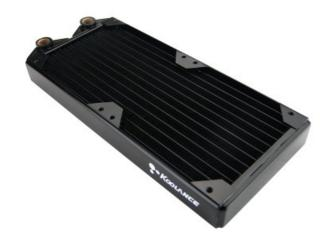
HX-CU720V is a low profile copper core radiator designed for two 120mm fans. With a fin density of 30 FPI (fins per inch), it offers best performance with higher air flow. It has a dual pass coolant design, and is G 1/4 BSPP (parallel) thread for hose fittings. 30mm (1.18") long mounting screws are included for 25mm thick fans (see Koolance <u>radiator screw packs</u> for additional options).
