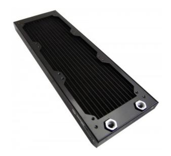
HX-1020 is a low profile aluminum radiator designed for two 120mm fans. With a fin density of 18 FPI (fins per inch), it is optimized for quieter air flow ranges. It has a dual pass coolant design, and is G 1/4 BSPP (parallel) thread for hose fittings. 30mm (1.18") long mounting screws are included for 25mm thick fans (see Koolance <u>radiator screw packs</u> for additional options).
