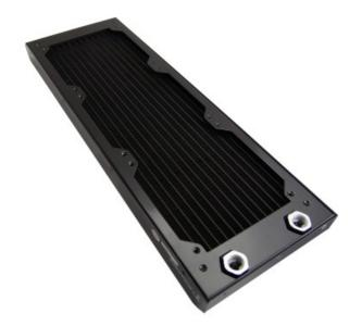
HX-1020 is a low profile aluminum radiator designed for three 120mm fans. With a fin density of 18 FPI (fins per inch), it is optimized for quieter air flow ranges, but will readily benefit from high CFM fans. It has a dual pass coolant design, with G 1/4 BSPP (parallel) threads for tube fittings. 30mm (1.18") long mounting screws are included for 25mm thick fans (see Koolance radiator screw packs for additional options).
