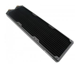
HX-CU1403V is a low profile copper core radiator designed for three 140mm fans. With a fin density of 30 FPI (fins per inch), it offers best performance with higher air flow. It has a dual pass coolant design, and is G 1/4 BSPP (parallel) thread for hose fittings. 30mm (1.18") long mounting screws are included for 25mm thick fans (see Koolance <u>radiator screw packs</u> for additional options).
