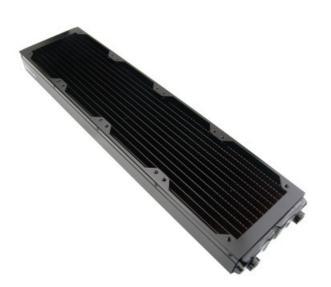
HX-480HL is a low profile copper core radiator designed for four 120mm fans. With a fin density of 11 FPI (fins per inch), it is optimized for quieter air flow ranges. It has a dual pass coolant design, and is G 1/4 BSPP (parallel) thread for hose fittings. 30mm (1.18") long mounting screws are included for 25mm thick fans (see Koolance <u>radiator screw packs</u> for additional options).
