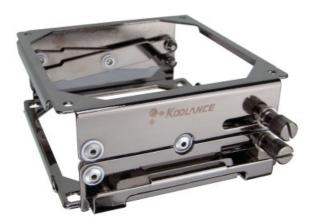
The Koolance BKT-HX001 is an adjustable heat exchanger mounting bracket with quick-release feature. Heavy steel construction supports heavier radiators (such as 4-fan sizes) with minimal movement. BKT-HX001 is designed for 120mm fan radiator spacing, with holes to mount to a 120mm fan grill on the computer chassis side.
