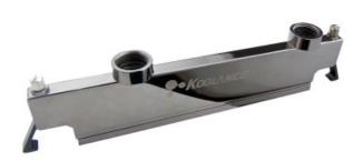
The full metal Koolance RAM-33 is among the most efficient liquid cooled memory product available. Koolance's (patent-pending) memory coolers physically run liquid along both sides of every DDR4, DDR3, DDR2, DDR, or SD DIMM. (Not compatible with FB-DIMM.) This occurs all the way down to the bottom of every chip!
