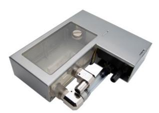
The RP-950 is a standalone reservoir and pump unit without electronic control or an LED display. It otherwise features identical components to the Koolance RP-1000 used in 1kW series systems. It features the powerful Koolance PMP-400 Pump integrated into a single 5.25" (CD) bay. The pump has a 3-pin connection (with tach lead), and a 3-4 pin 12V Molex power adapter is included for easy connection to a power supply.
