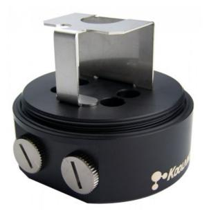
Acetal fitting base for Koolance 80mm OD reservoir bodies. Redundant inlet and outlets are provided for inline or parallel loops. Two nickel-plated brass socket plugs, a reservoir oring, and removable stainless steel partition are included.
