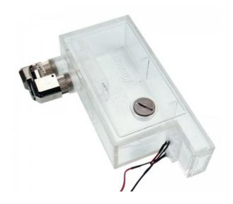
Reservoir used in the Koolance RP-1000 and RP-1005 products, usually combined with the PMP-400 pump. Includes blue LED tank lighting. Swiveling fittings are 3/8in (10mm) ID, nickel-plated brass. Overall size including fittings is 4.4" x 6.1" x 1.6" (11.2cm x 15.5cm x 4cm).
