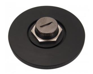
Acetal reservoir top for Koolance <u>60mm OD reservoir bodies</u>. Nickel-plated brass, G 1/4 BSPP (parallel) thread top fill port. Hex mounting nut and insulating washer included.
