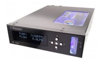
The RP-1250 is a combined reservoir and pump unit which fits into a single 5.25" (CD) bay. Featuring the powerful Koolance PMP-400 pump, it also includes temperature monitoring, a front display, reservoir, pump & fan speed control, and rear G 1/4in threaded fitting sockets. This unit incorporates all-new Koolance electronics, with a 2-line OLED display for deeper user control and feedback.
