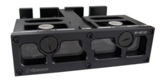
Easily combine Koolance's compact high pressure pumps into dual or serial/redundant loops! RP-401X2 is a single 5.25" bay reservoir designed for **one or two** Koolance PMP-400 pumps (not included). Using a convenient bottom plug, the front reservoirs can be separated or combined without disassembling the unit. Top fill ports are available for each reservoir.
