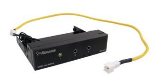
The Koolance SEN-LK001 offers leak detection for very small amounts of water. Housed in a 3.5in drive bay profile, the electronic circuit can monitor up to three separate leak sensing cables. One 46cm (18in) long sensing cable is included, which can be increased. Powered by 12VDC from a computer power supply connection.
