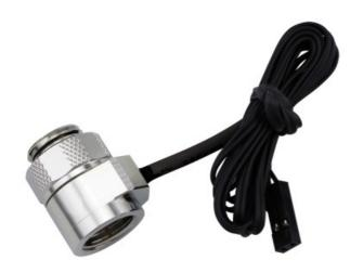
Coolant thermistor temperature sensor within a swiveling brass body. Male and female G 1/4 BSPP threads are provided on either end. Wire length = 30" (76cm). NOTE: This sensor will only work with Koolance products which use 10K Ohm @25°C sensors (first introduced in 2011).
