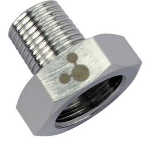
Single fitting threading adapter, from NPT 1/8 (male) to G 1/4 BSPP (female).
