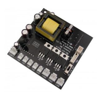
The TMS-EB205 Expansion Board doubles the amount of components which <u>TMS-205</u> can monitor and control. Added features include:
