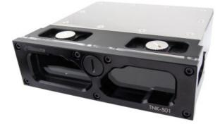
TNK-501 is a single 5.25" bay reservoir. Machined from a solid piece of acetal for maximum reliability, it has a thick acrylic window, front aluminum bezel, and stainless steel top cover. TNK-501 features 8 total G 1/4 BSPP (parallel) thread sockets: 2 on top, 2 on bottom, and 4 on the back. 6 socket plugs are included.
