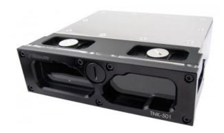
TNK-501 is a single 5.25" bay reservoir. Machined from a solid piece of acetal for maximum reliability, it has a thick acrylic window, front aluminum bezel, and stainless steel top cover. TNK-501 features 8 total G 1/4 BSPP (parallel) thread sockets: 2 on top, 2 on bottom, and 4 on the back. 6 socket plugs are included.
