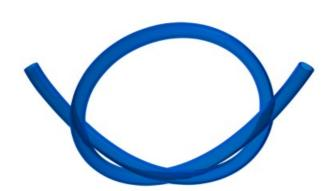
Koolance blue PVC tubing with 13mm (1/2in) internal diameter, 16mm (5/8in) external diameter. Bend radius is approximately 55mm (2.2in). This tubing is priced per foot (305mm) and will be cut to the ordered length.
