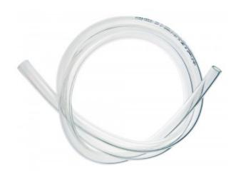
Koolance clear PVC tubing with 10mm (3/8in) internal diameter, 13mm (1/2in) external diameter. Length 15m/ 49.2ft. Bend radius is approximately 37mm (1.5in).
