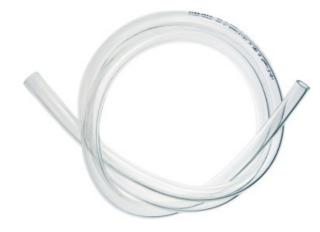
Koolance clear PVC tubing with 10mm (3/8in) internal diameter, 13mm (1/2in) external diameter. Length 15m / 49.2ft. Bend radius is approximately 37mm (1.5in).
