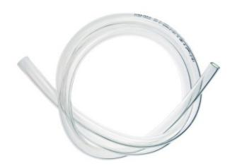
Koolance clear PVC tubing with 10mm (3/8in) internal diameter, 13mm (1/2in) external diameter. Length 3m / 9.8ft. Bend radius is approximately 37mm (1.5in).
