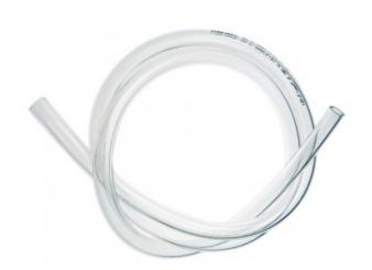
Koolance clear PVC tubing with 13mm (1/2in) internal diameter, 16mm (5/8in) external diameter. Length 15m / 49.2ft. Bend radius is approximately 55mm (2.2in).
