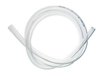
Koolance clear PVC tubing with 13mm (1/2in) internal diameter, 16mm (5/8in) external diameter. Length 15m / 49.2ft. Bend radius is approximately 55mm (2.2in).
