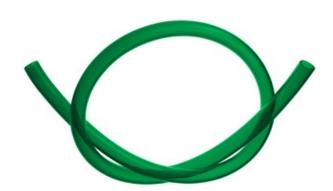
Koolance green PVC tubing with 10mm (3/8in) internal diameter, 13mm (1/2in) external diameter. Bend radius is approximately 37mm (1.5in). This tubing is priced per foot (305mm) and will be cut to the ordered length.
