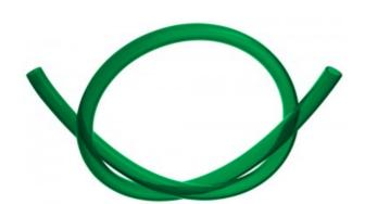
Koolance green PVC tubing with 13mm (1/2in) internal diameter, 16mm (5/8in) external diameter. Bend radius is approximately 55mm (2.2in). This tubing is priced per foot (305mm) and will be cut to the ordered length.
