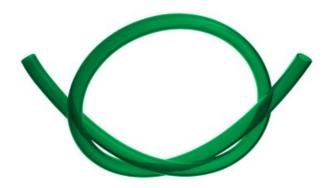
Koolance green PVC tubing with 13mm (1/2in) internal diameter, 16mm (5/8in) external diameter. Bend radius is approximately 55mm (2.2in). This tubing is priced per foot (305mm) and will be cut to the ordered length.
