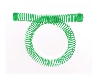
Tubing outer spring to help avoid kinks in tight areas. Steel with green plastic coating. For 13mm (1/2in) external diameter tubing.
