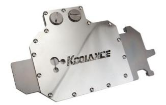
The new Koolance VID-428 is a combined GPU and memory cooler for high-end video cooling of GeForce GTX 280 and GTX 260 (65nm) cards in single or multi video configurations. It combines a full nickel-plated solid copper cooler which targets all primary heat-producing regions of the GTX 280/260 (including the voltage regulators). An acrylic lid allows coolant visibility under the logo. A rear memory heat sink plate is also included.
