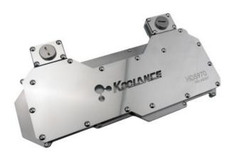
The Koolance VID-AR597 is a combined GPU and memory block for high-end water cooling of ATI Radeon HD 5970 2GB video cards in single or multi video configurations. It combines a full nickel-plated solid copper cooler which targets all primary heat-producing regions of the HD 5970 (including the voltage regulators). An acrylic lid allows coolant visibility under the logo.
