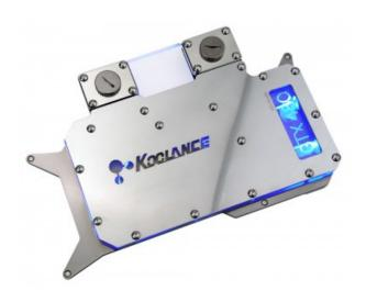
The Koolance VID-NX480 is a combined GPU and memory block for water cooling NVIDIA GTX 480 video cards in single and multi video configurations. It utilizes a high-performance microfin design (0.5mm) made of solid copper with anti-corrosive nickel plating. The cooler targets all primary heat-producing regions of the GTX 480, including the voltage regulators. The top stainless steel cover plate protects an LED illuminated acrylic lid.
