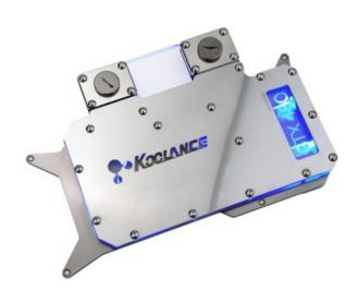
The Koolance VID-NX480 is a combined GPU and memory block for water cooling NVIDIA GTX 480 video cards in single and multi video configurations. It utilizes a high-performance microfin design (0.5mm) made of solid copper with anti-corrosive nickel plating. The cooler targets all primary heat-producing regions of the GTX 480, including the voltage regulators. The top stainless steel cover plate protects an LED illuminated acrylic lid.
