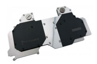
The Koolance VID-NX590 is a full coverage video block for water cooling NVIDIA GeForce GTX 590 cards in single and multi video card configurations. It utilizes a high-performance microfin (0.5mm) design made of solid copper with anticorrosive nickel plating.
