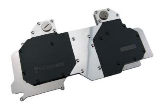
The Koolance VID-NX590 is a full coverage video block for water cooling NVIDIA GeForce GTX 590 cards in single and multi video card configurations. It utilizes a high-performance microfin (0.5mm) design made of solid copper with anti-corrosive nickel plating.
