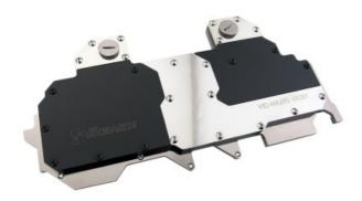
The Koolance VID-NX690 is a full coverage video block for water cooling NVIDIA GeForce GTX 690 cards in single and multi video card configurations. It utilizes a high-performance microfin (0.5mm) design made of solid copper with anticorrosive nickel plating.
