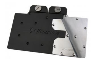
The Koolance VID-AR290X is a full coverage video block for water cooling AMD Radeon R9 290 and 290X cards in single and multi video card configurations. It utilizes a high-performance microfin (0.5mm) design made of solid copper with anti-corrosive nickel plating.
