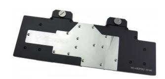
The Koolance VID-AR295X2 is a full coverage video block for water cooling AMD Radeon R9 295X2 cards in single and multi video card configurations. It utilizes a high-performance microfin (0.5mm) design made of solid copper with anti-corrosive nickel plating.
