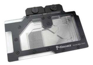
The Koolance VID-NX1080 is a full coverage video block for water cooling NVIDIA reference GeForce GTX 1080 and GTX 1070 cards in single and multi video card configurations. It utilizes a high-performance microfin (0.5mm) design made of solid copper with anti-corrosive nickel plating. This version has an acrylic top with holes for LED lights (not included). Thermal interface material and mounting hardware are included. Tube fitting threads are G 1/4 BSPP.
